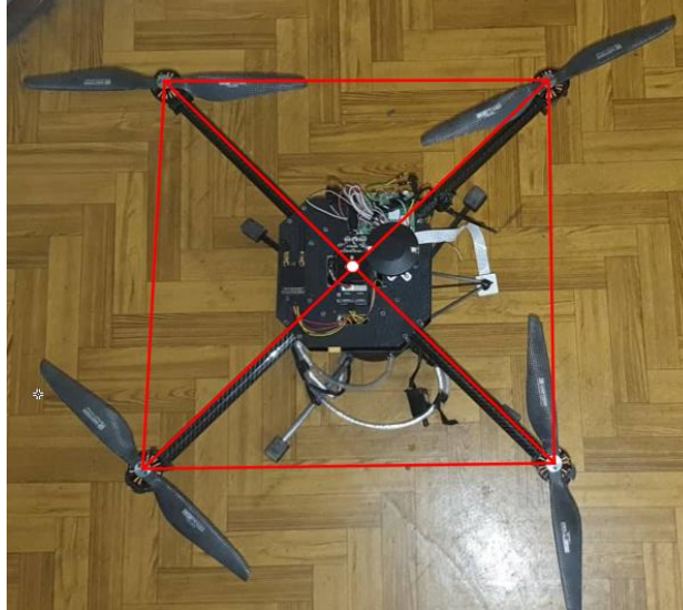
Figure 1. Determination of the centre of gravity of the drone.
